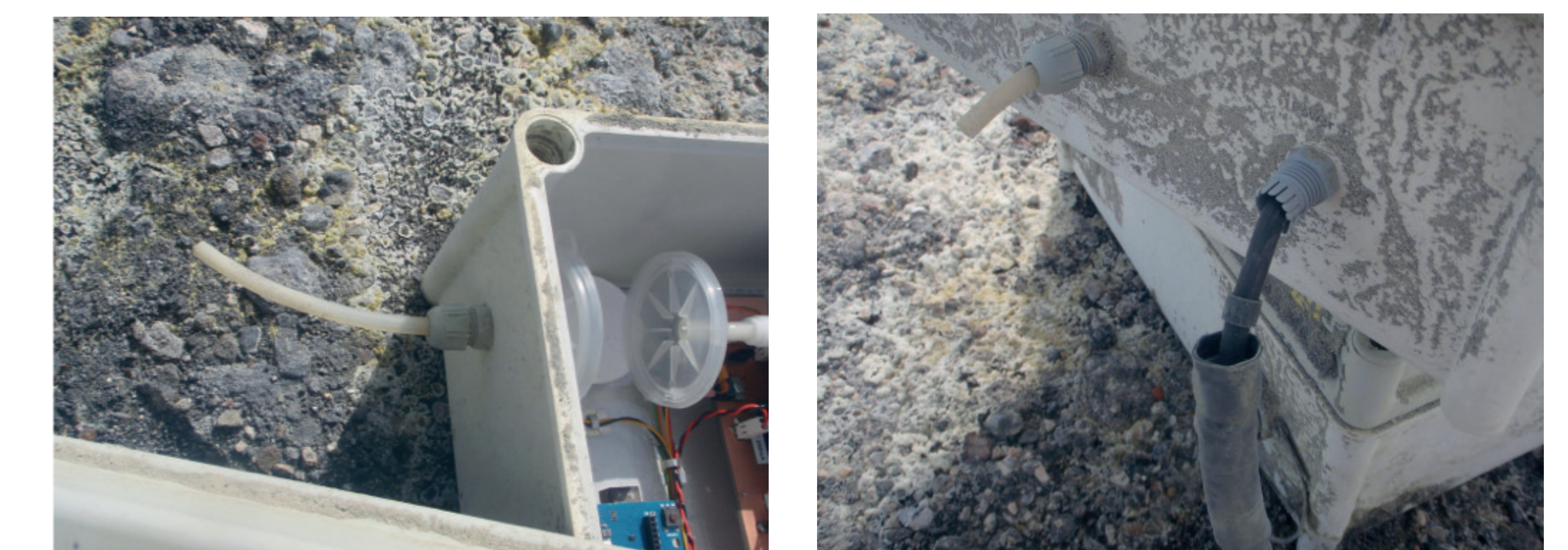
Photos of the vandalised PT-1A prototype. [LEFT] Tugging on the gas inlet resulted in the filter disconnecting [RIGHT] The armoured cable between the power and sensor boxes was damaged.
